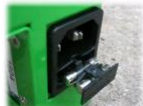
IEC power socket showing fuse access
